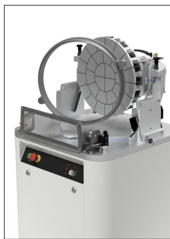
2. Remove the ring and clean it inside with a plastic scraper
